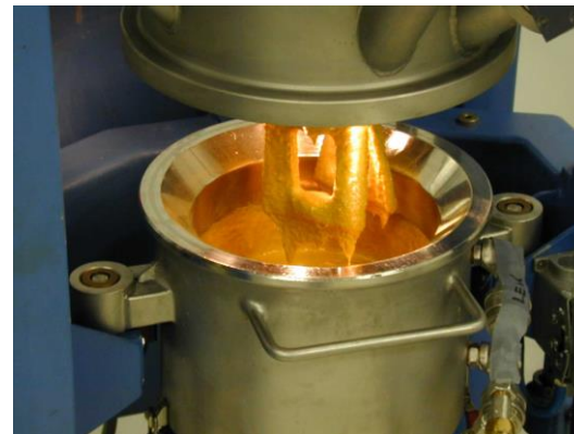
HKV5 mixer, double planetary mixer, max. 4-5 kg
