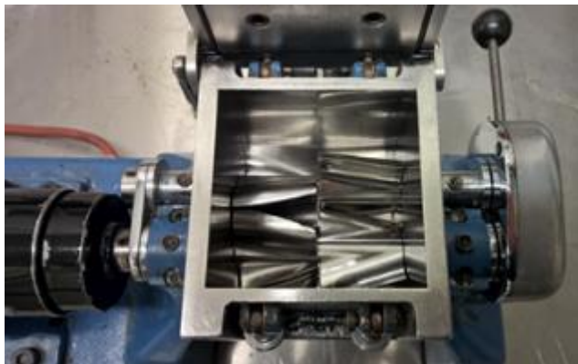
IKA high shear mixer, horizontal mixing blades, max. 350 g
